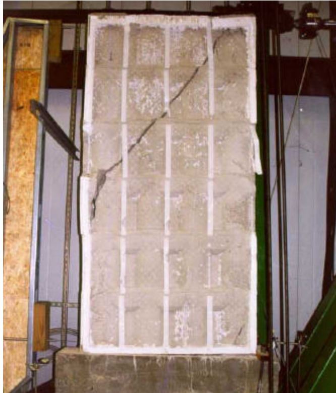
Figure 7 Failure Mechanism of Waffle No. 1 Wall Specimen
