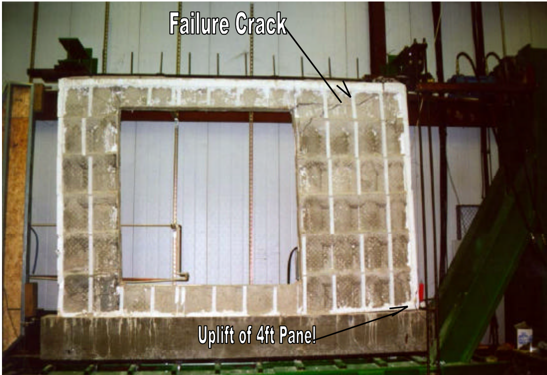
Figure 9 Failure Mechanism of Waffle No. 2 Wall Specimen
