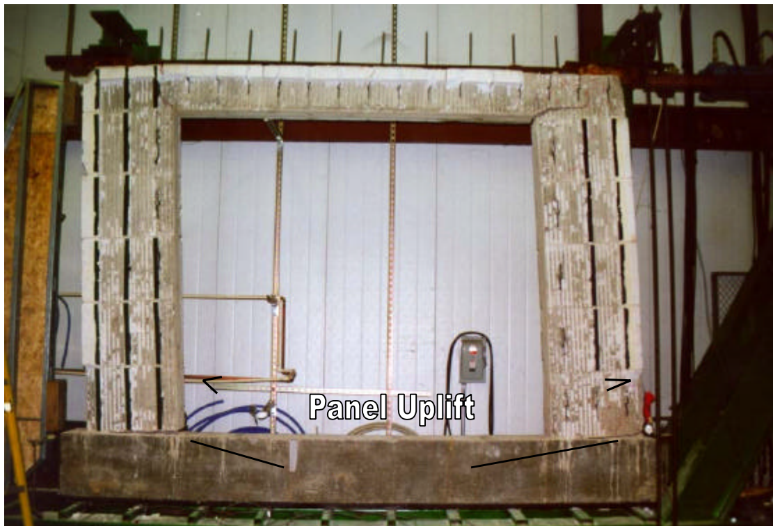
Figure 6 Final Lateral Displacement of Flat No. 3 Wall Specimen
