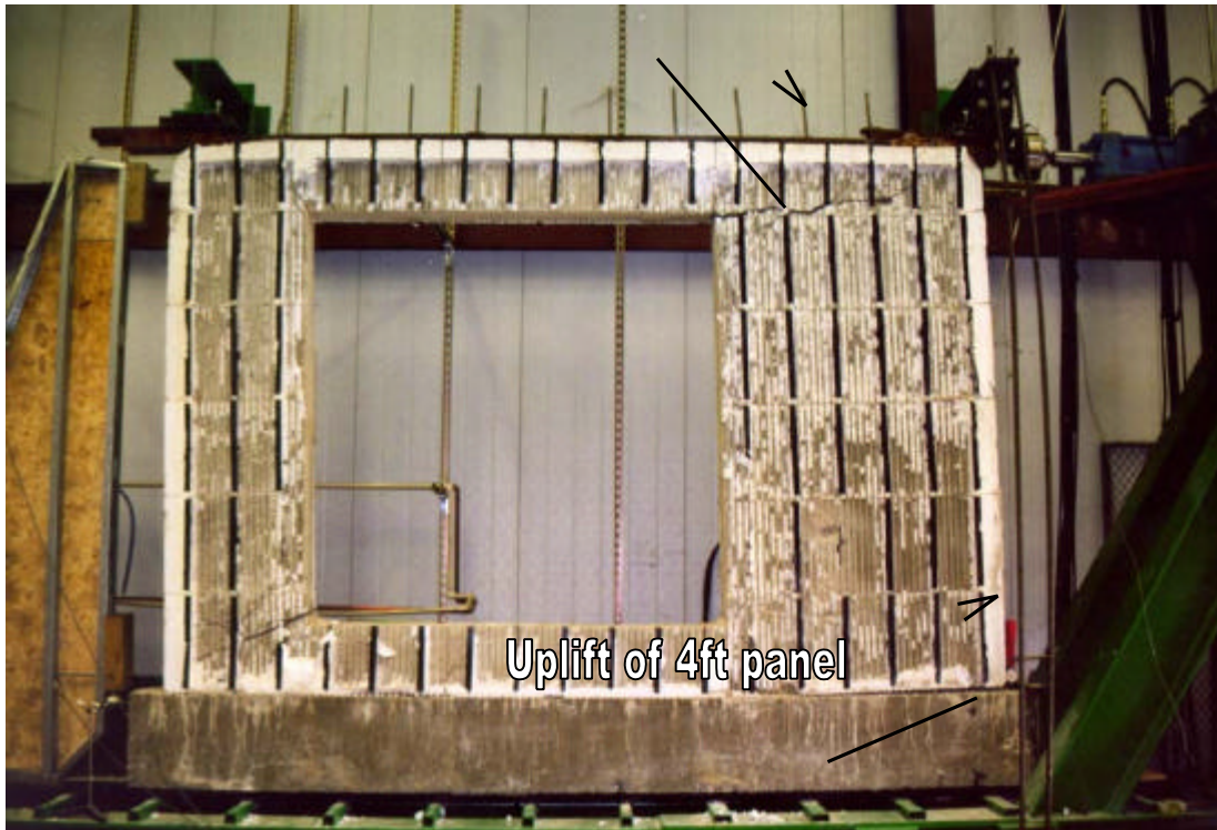
Figure 4 Failure Mechanism of Flat No. 2 Wall Specimen
